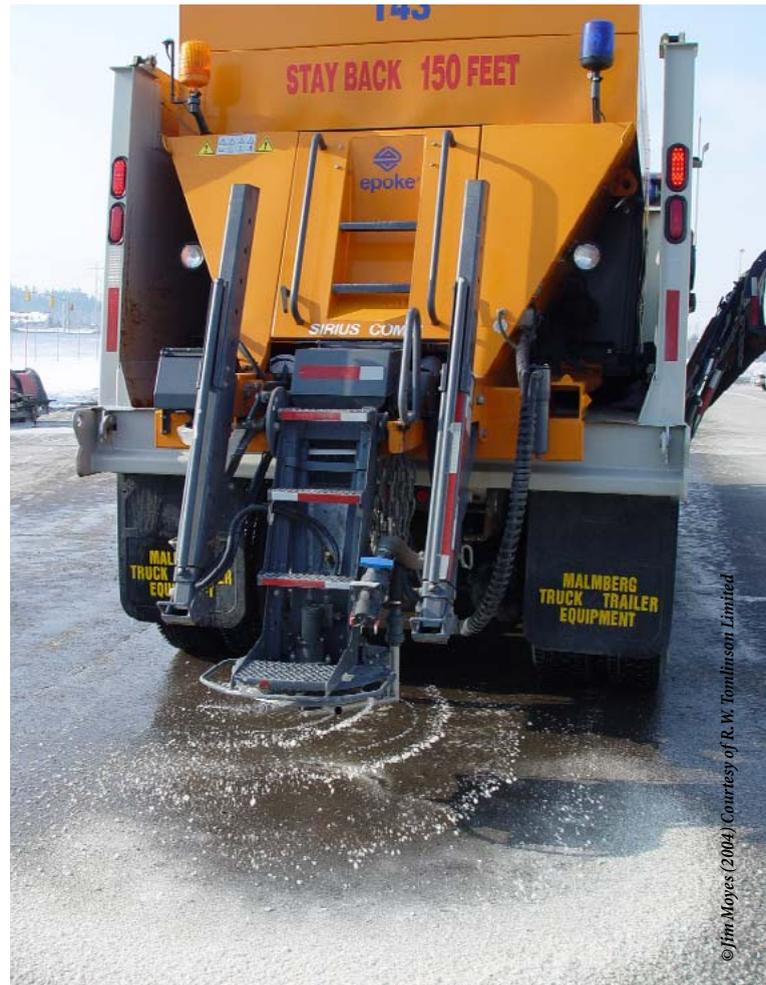
*New model salt spreader hard at work.*
